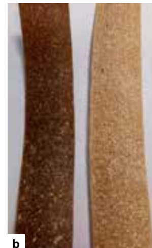
(a) Twin screw extruder enables the elaboration of new biomaterials, the extraction of molecules of interest from biomasses and reactive extrusion to be carried out by adding various reagents and enzymes. It's a versatile tool calibrated for research and scale-up. (b) example of a new biocomposite produced with agro-industrial by-products to substitute traditional plastics.
